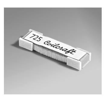
The 5315TC is Coilcraft's most rugged and lowest cost antenna coil designed for RFID applications at 125 kHz. The wrap-around terminals have large mounting surfaces to ensure excellent board adhesion. The coil is wound on a plastic base, providing great durability and allowing this part to withstand harsh mechanical shock.
